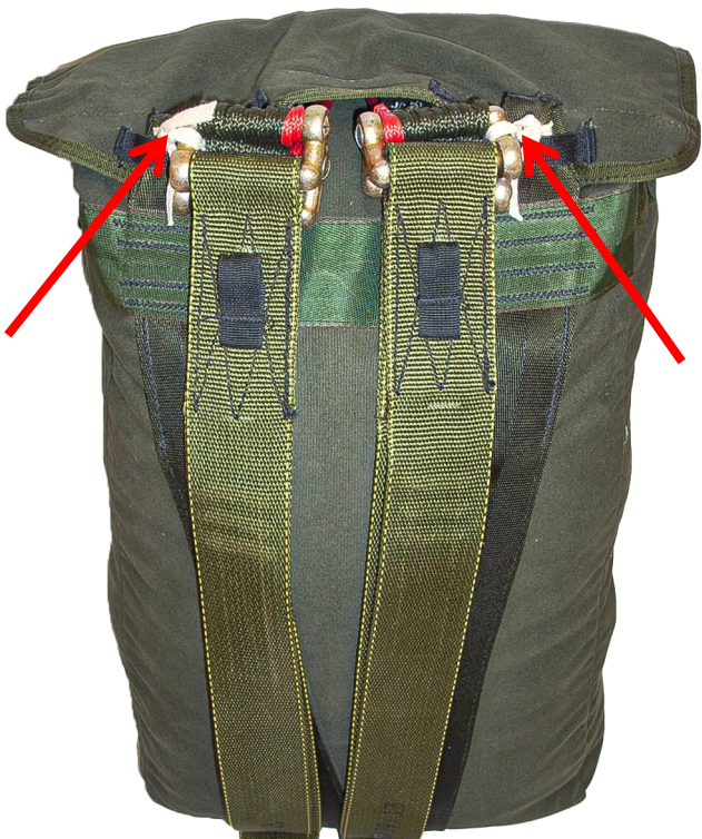
Riser to Deployment Bag 80 lbs. Break-tape
