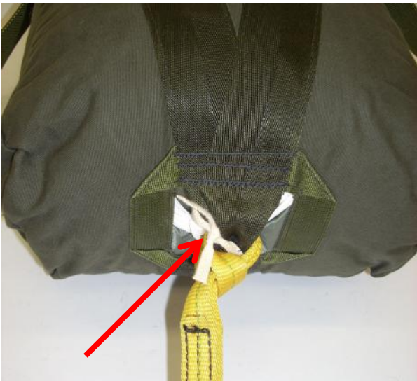
80 lbs. Break-tape Canopy to Deployment Bag Attachment
