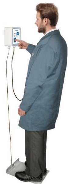
Testing static dissipative shoes before entering hazardous area
