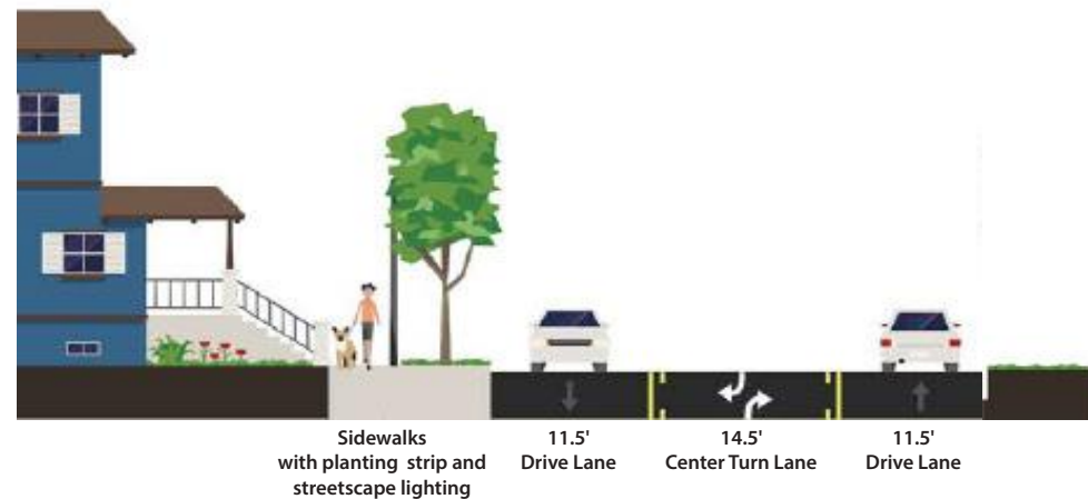
Figure 53: St. Louis Road design with proposed roadway configuration, sidewalk, shared use path, and streetscape improvements
