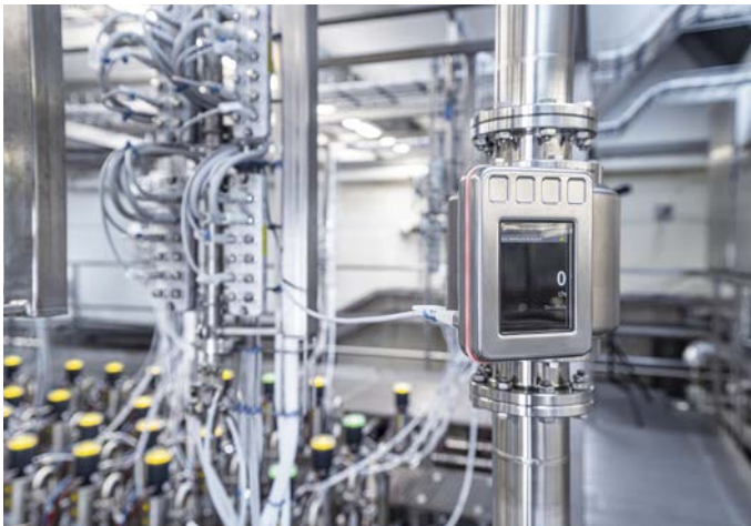
EvoConnect control tops and measurement devices are fully integrated into the digital control system via IO-Link.
