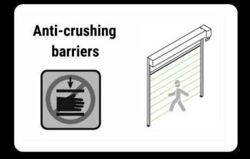
There is a safety light curtain integrated on the legs. When it detects an obstacle it inverts the direction of the curtain.
