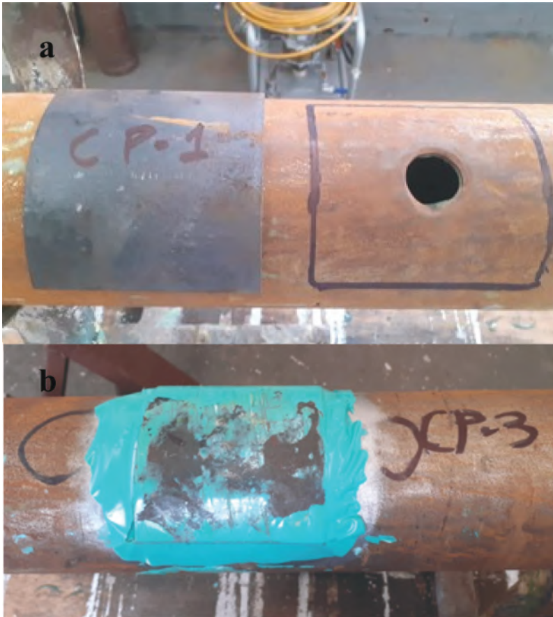
Figure 1. Curved plate and pipe used in the test (a) and curved plate bonded to the pipe (b).
