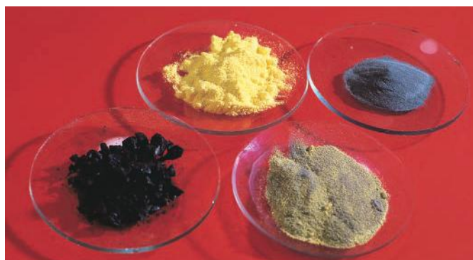
▲ Figure 2.8 The elements sulfur and iron at the top of the photograph, and (below) black iron(II) sulfide on the left and a mixture of the two elements on the right
