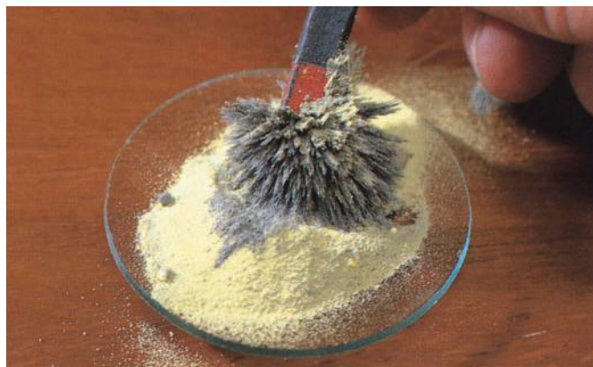
▲ Figure 2.9 A magnet will separate the iron from the mixture
