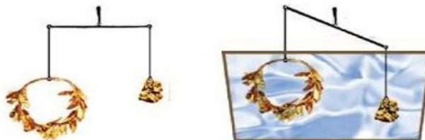
Figure 17: When balanced, Archimedes' crown and the pure gold had the same mass, but the crown displaced more water. It had a higher volume than the real gold, proving it wasn't real!
