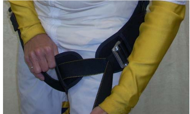
Adjusting the Leg Straps.
