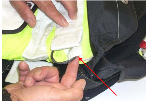
Tuck any excess RSL into the channel pocket on the top left side of the free-bag.
