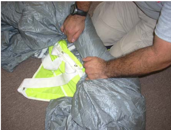
Roll the center material to the depth of the Free-bag. Place your knee on to hold in place.
