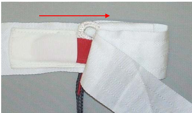
Stow the Spectra Line Loop into the looped polyester sleeve opposite the long pin channel.
