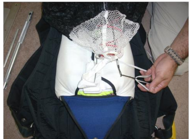
Pull the pull-up cord through the Pilot chute.
