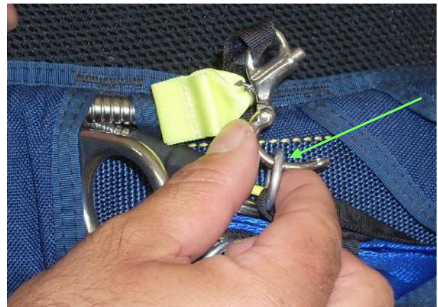
Attach the Shackle to the Reserve Static Line (RSL) ring.
