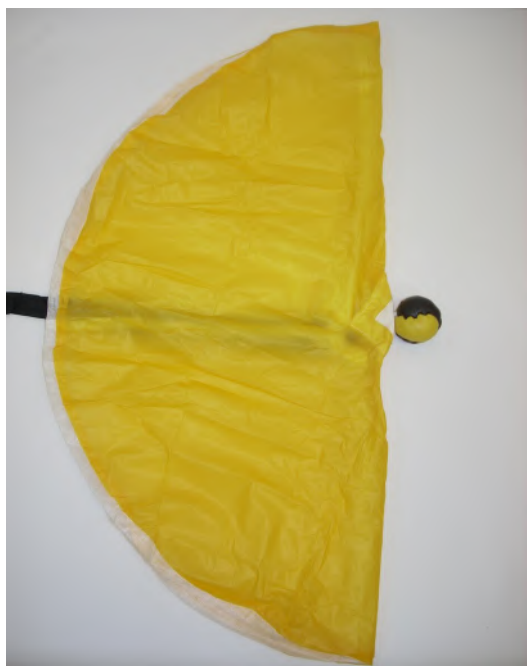
Fold the Pilot chute in 1/2 with the bridle coming out of the middle.
