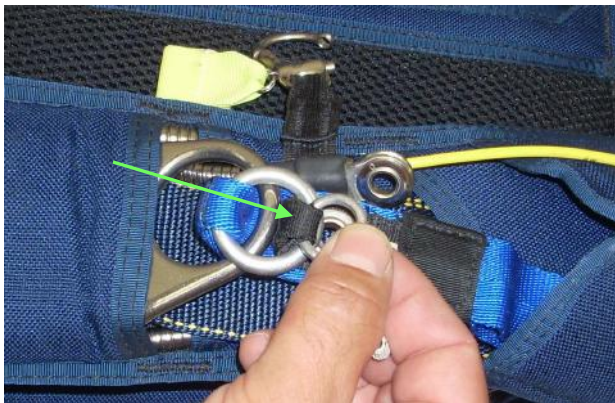
Pass the small ring of the Riser through the large ring of the Riser .
