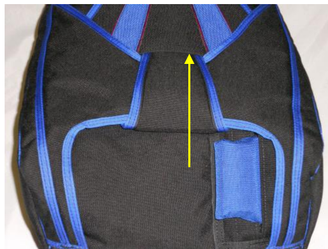
Close the Main Pin Protector Flap.
