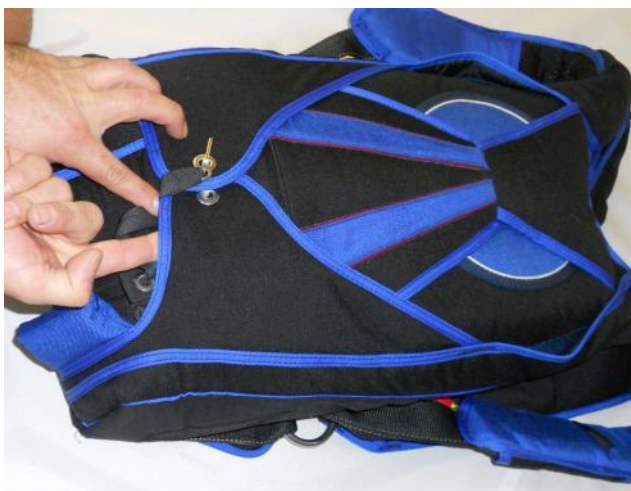
Tuck the extra Pull-out Bridle under the Right Side Flap.
