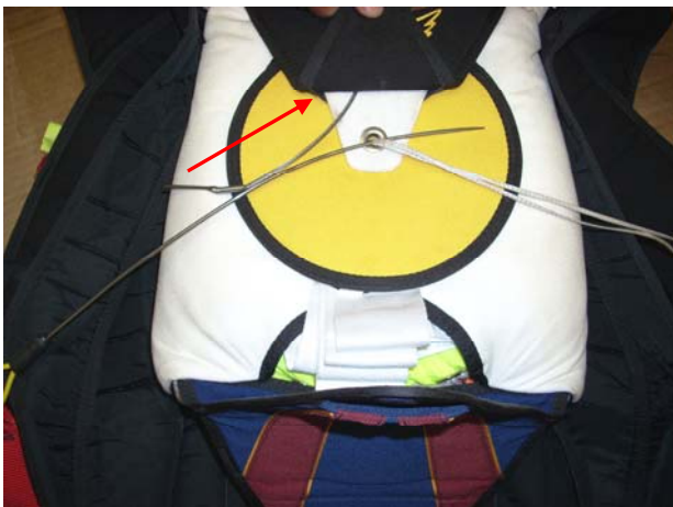
Make sure the Top Closing Flap is under the retaining tape of the Top Pin Cover Flap. Close and secure with a temporary pin.
