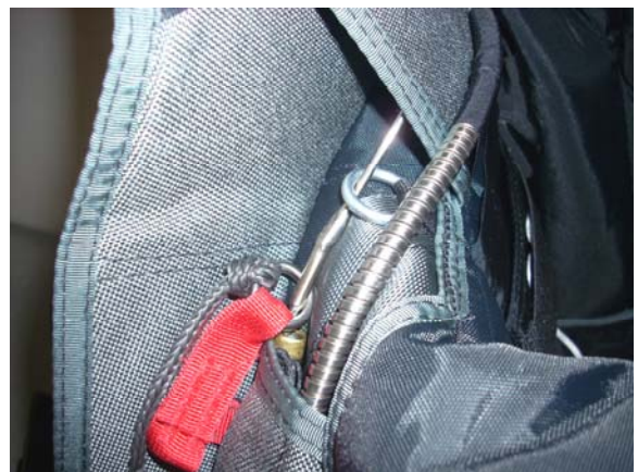
Open up the Reserve Container. Check to be sure that the Reserve Static Line is installed correctly. If using a M.A.R.D. "Reserve Boost" be sure that you are using a M.A.R.D. "Reserve Boost" RSL and that the Reserve Ripcord cable passes through the middle ring of the RSL.
