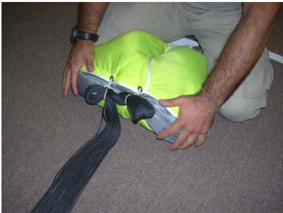
Use two (2) line bights @ 1 1/2" -2" to secure the Free-bag closed.
