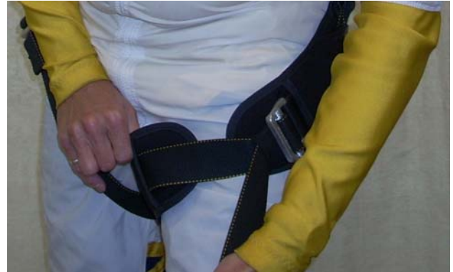
Adjusting the Leg Straps.
