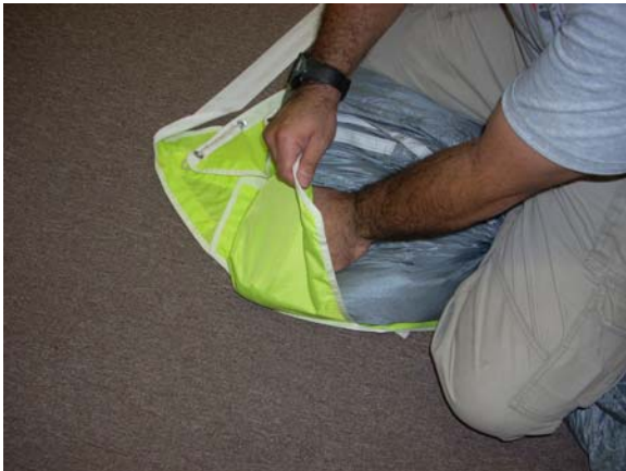
Tuck the canopy into the corners of the Free-bag.
