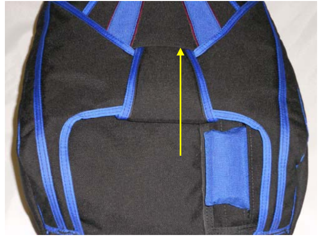
Close the Main Pin Protector Flap.
