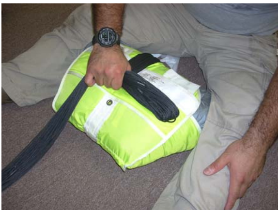
Begin to stow the rest of the reserve parachute lines into the pocket on the Free-bag.
