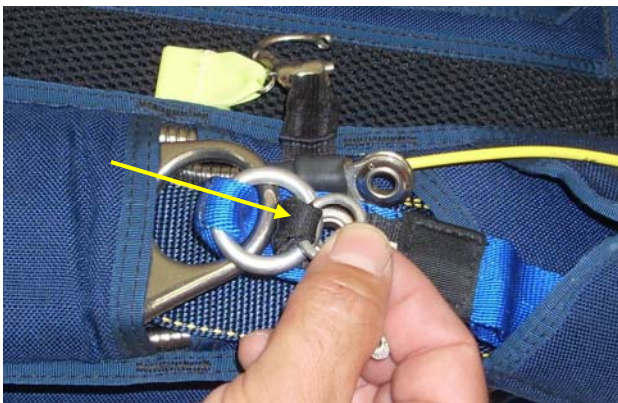
Pass the small ring of the Riser through the large ring of the Riser .
