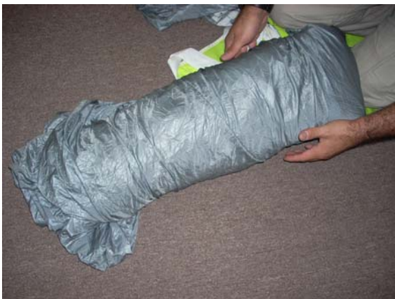
Straighten and smooth out the "ear" formed after following the center seam.
