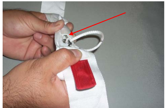
Slide the Long Pin through the loop then stow into the channel under the tuck tab channel. Be certain that it is in its own channel.
