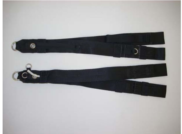
TPDS-MIS-204 Main Risers T-8
