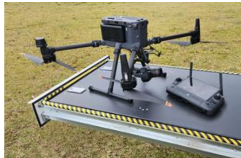
LiDAR drone for capturing images. Photo: NRAR
