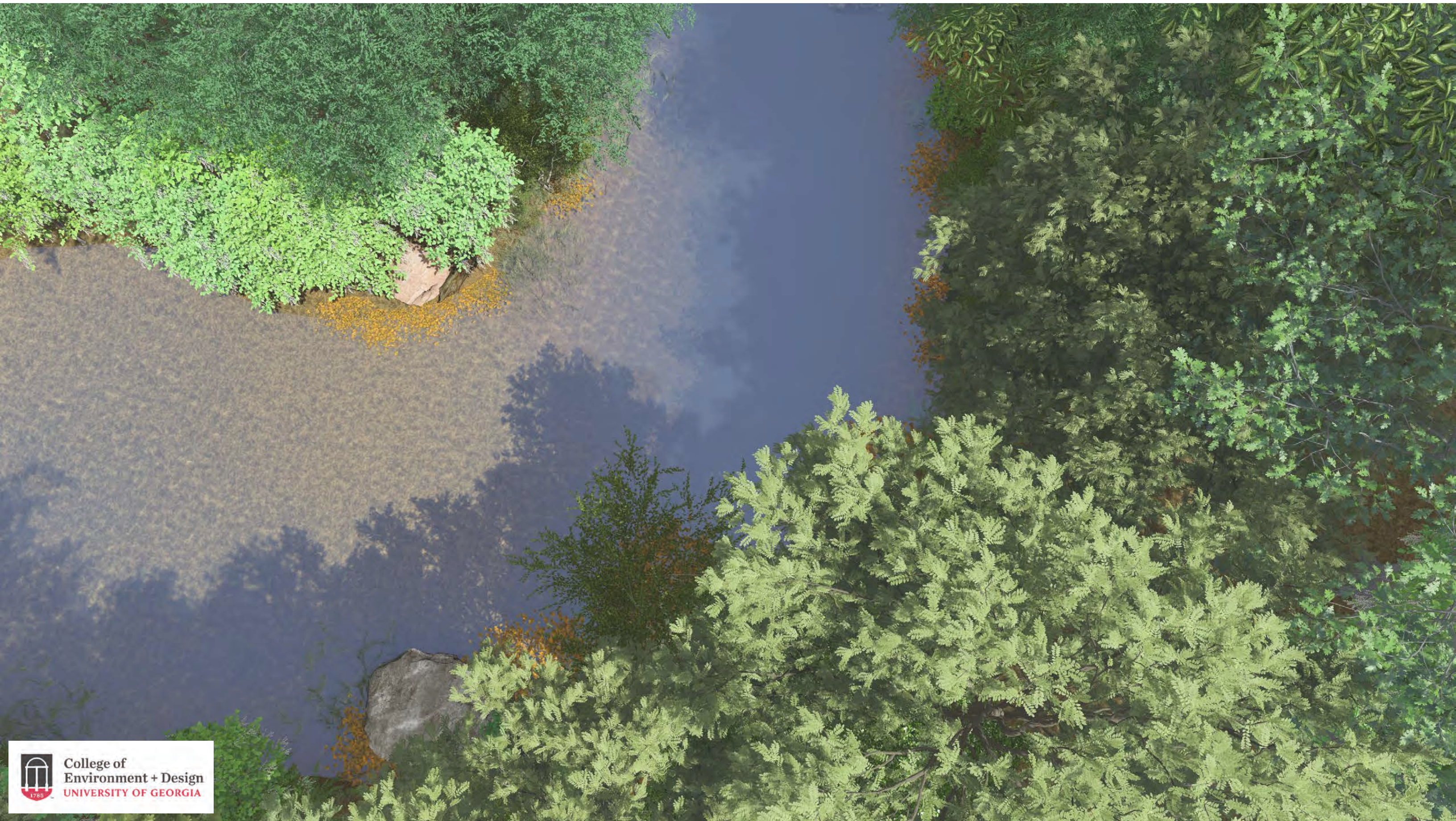
Increased sinuosity in the design re-directs the stream to wind through the landscape, slowing its flow.
