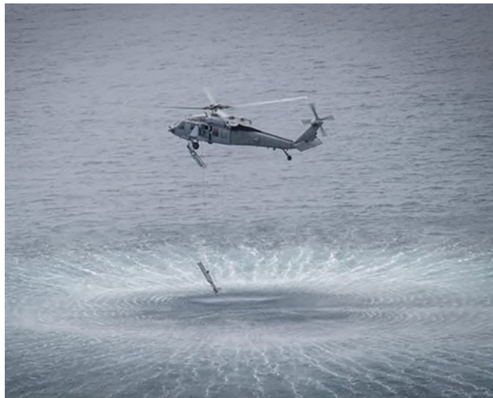
An MH-60S from HSC-21 lowers AMNS gear into the water to conduct MCM operations against mine contacts found by HM-14 and HM-15 Sonar. U.S. Navy photo by MC1 Sara Eshleman.
