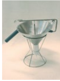
M1122 Dosing funnel Ideal for dosing jelly and liquid ganaches 1,2 litre Ø 185 x 210 mm Manual control Stainless steel made, nozzles, dosing head and handle are made out of plastic Ø nozzles: 4 and 8 mm Holder not included
