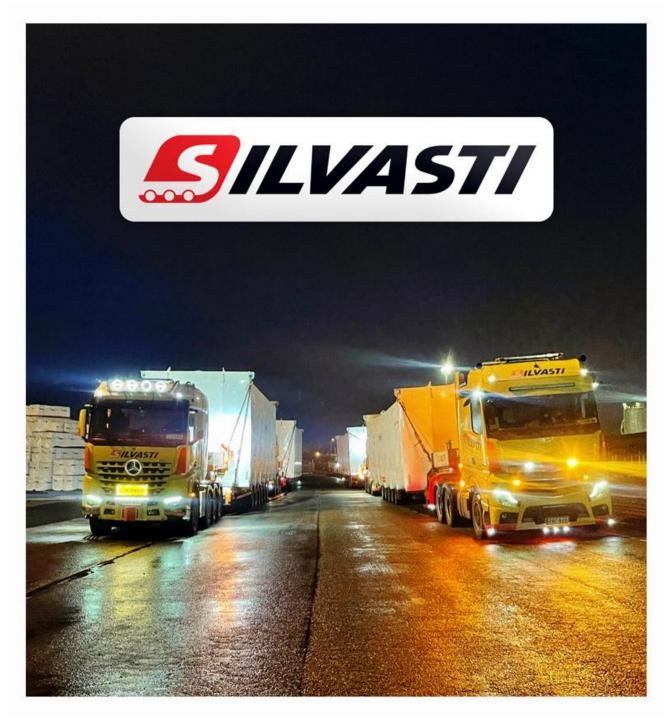
Wide transport on the road! This 6,5 meters wide and 5,5 meters high technical building module was transported from Finnish Ostrobothnia to Northern Sweden.
