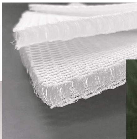
Microripstop nylon 100% PA 53 gsm
