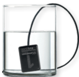
Waterproof & fully submersible for optional infection control
