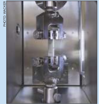
Crack-bridging test according to EN 14891: Waterproofing membranes formulated with VINNAPAS® 754 ED and VINNAPAS® 764 ED can compensate for cracks even at temperatures below freezing, thus reliably protecting the building from water penetration.
