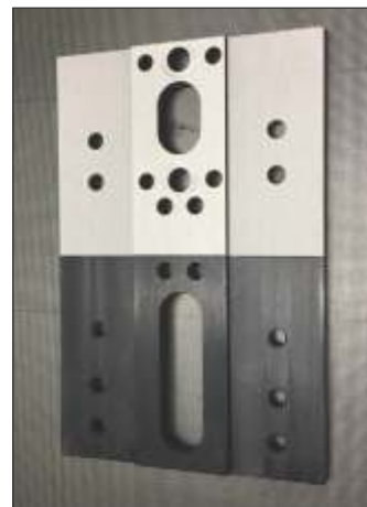
Laser systems remove corrosion, grease, residue, and existing coatings from metal surfaces quickly.
