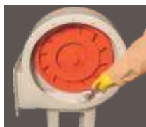
Inner Base of Dust Collector Coated with Aluma Coat - TW
