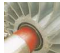
Motor Shaft Coated with Aluma Coat - BR
