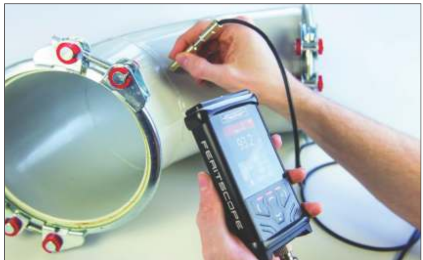
FERITSCOPE® DMP30: Instrument for measurement of the ferrite content in austenitic and duplex steel.
