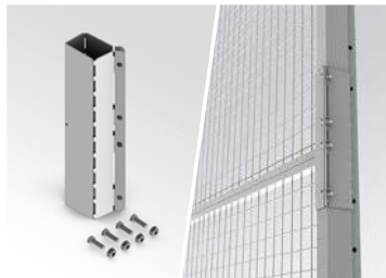
5 EXTENSION BRACKETS These brackets are a smart solution for taller Partitioning walls. Top fixings are recommended when building above 4,400 mm.
