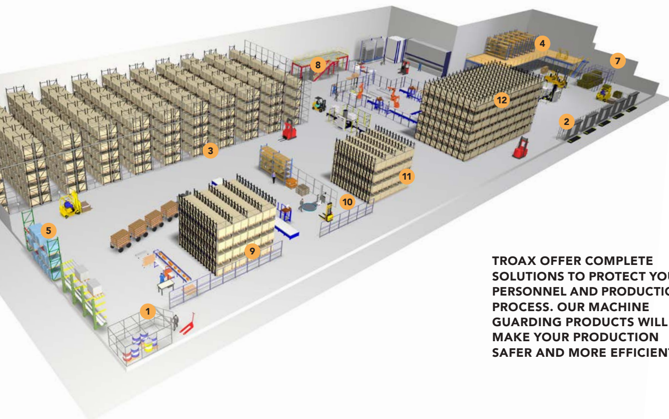
4 MEZZANINE GUARD The Mezzanine system with posts, panels, kick plates and guard rail protects both people and loose objects from falling down.
