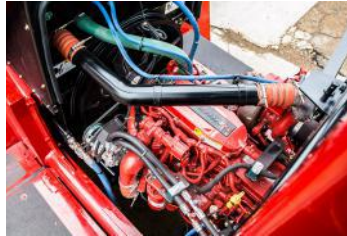
Easy Access to Drive Train & Hydraulics
