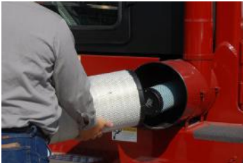
Donaldson Air Cleaner with Safety Element (Standard)
