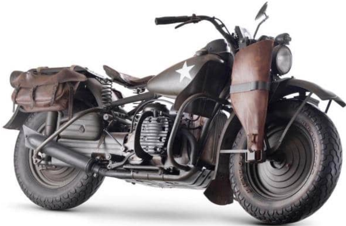
Harley-Davidson XA transverse flat twin complete with plunger rear suspension. Its springer fork was subsequently replaced with Harley-Davidson's first telescopic fork; a few were supplied with solid disc wheels.
