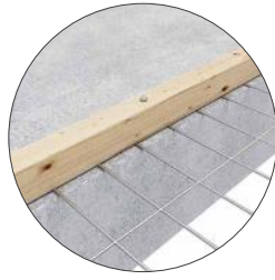
timber batten 40 x 50 mm
