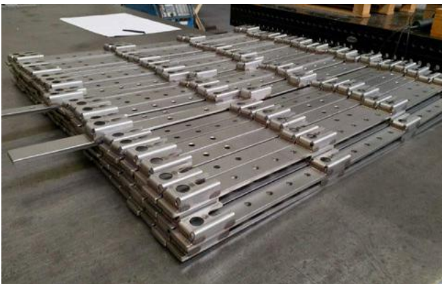
Production of the strips with mounted filler blocks
