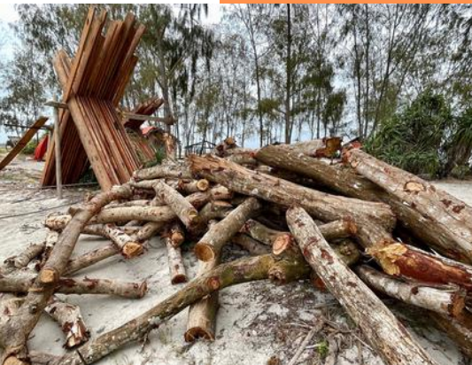
Mangrove trunks and Alamendra (sea almond) logs drying for use as frames for dhows; natural curved pieces are selected to fit the shape of the hull.
