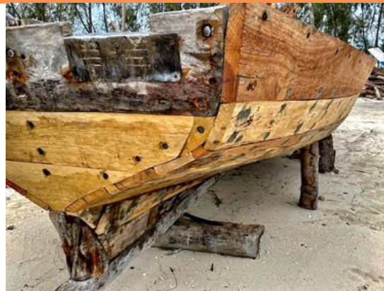
Planking, transom, keel details. Iron spikes are visible. They are wrapped with cotton caulking before they pound them into the planking and counter sink. Later, seam compound and paint is applied to seal.
