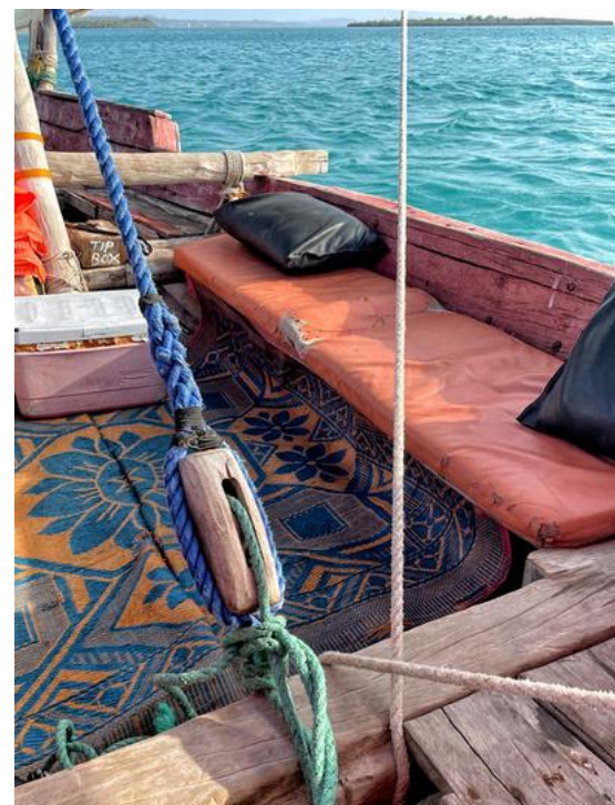
The main halyard aboard MAPENZE serves as the primary shroud and back stay when under sail.
