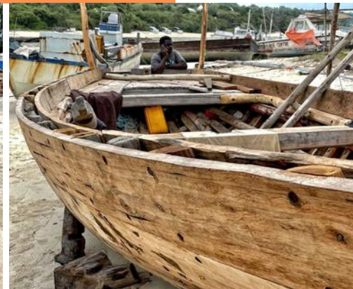
Mahogany planking fastened to almond or mangrove heavy frames with hand-drilled holes and tree nails or 5-inch iron spikes, then hammered over on the inside of the frames.
