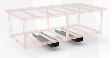
FORKLIFT SLOTS PART NO. 5610330
