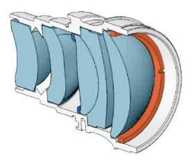
RPO's expertise in precision assemblies, glass and plastic hybrid designs, and high-volume production can cut cost, reduce weight, and improve performance.
