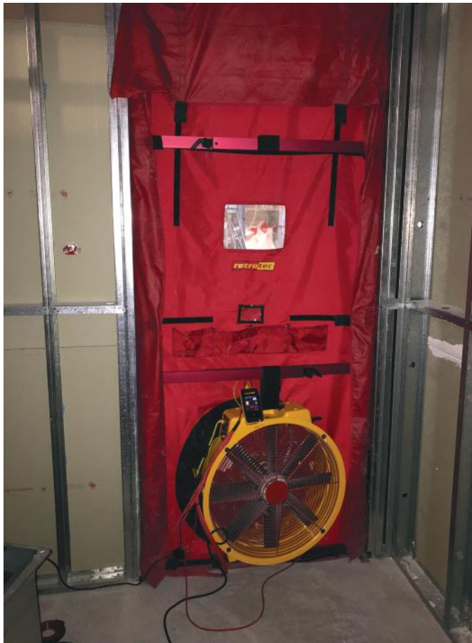
Figure 8: Building Pressure Test - Testing Setup
