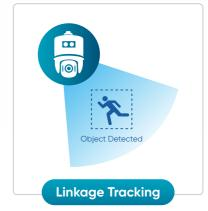
When an object enters the view of the static lens, the PTZ lens is automatically triggered to track it.
