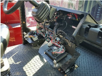
Flip-down Dash with Color/Number Coded Wiring (Standard)
