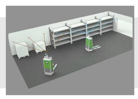
The Palletmover utilizes natural navigation with top-mounted laser scanning to ensure precise and reliable movement.
