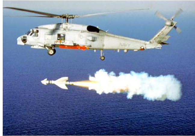
During operational testing, an AGM-119B Penguin anti-ship missile heads toward its target after being fired. Photo from the U.S. National Archives.
