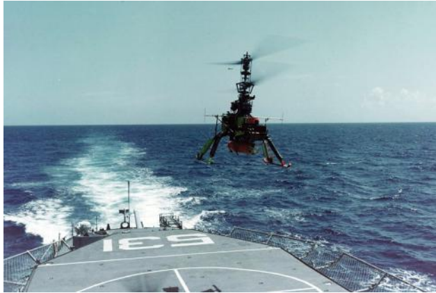
DASH (Drone Anti-Submarine Helicopter) the U.S. Navy's new long range anti-submarine weapon system. DASH hovers in free flight over the flight deck of USS Hazelwood (DD 531).
