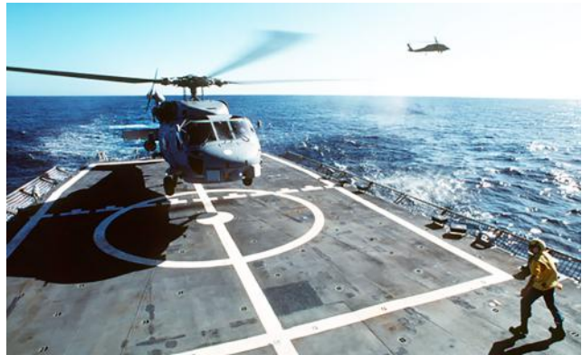
The Navy's first operational LAMPS (Light Airborne Multi-Purpose System) Mark III SH-60B Seahawk helicopter lifts off from the flight deck of the guided missile frigate USS Crommelin (FFG 37), during flight deck landing qualifications off the coast of San Diego. NARA/Getty Image.
