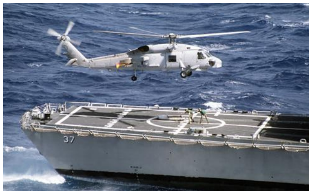
An SH-60B Sea Hawk Light Airborne Multipurpose System (LAMPS III) helicopter, from HSL-43, in flight near the stern of the guided missile frigate USS Crommelin (FFG 37). The helicopter is equipped with AN/ASQ-81 magnetic anomaly detection (MAD) gear.
