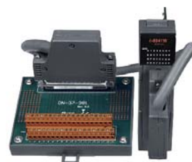
I-87024DW, I-87017DW with DN-37-381-A and DB37 Male to Female Cable (Optional)
