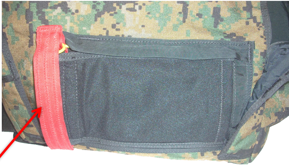
AFF Jumpmaster Handle for Throw-out Pilot-chute
