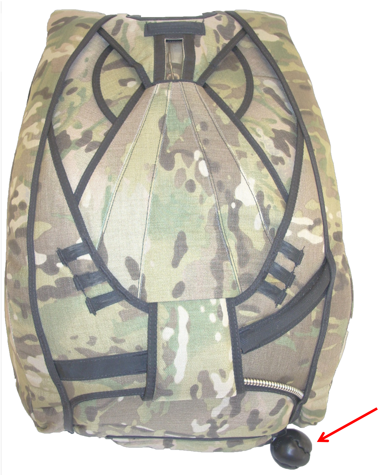
Throw-out Pilot-chute with Hacky Handle on BOC
