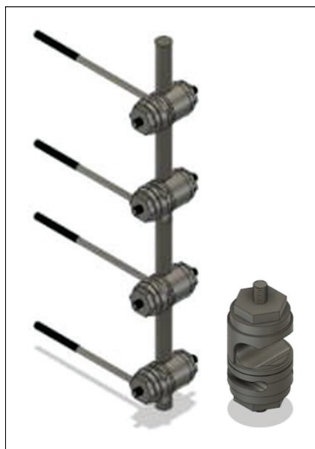
Figure 1. Single-rod modular external fixator prototype 3D render design.
