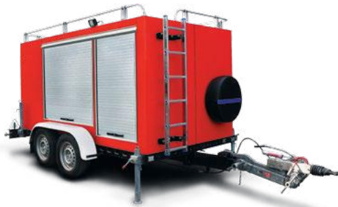
PUMPENANHÄNGER TRAILER WITH DRY POWDER EXTINGUISHING UNIT
