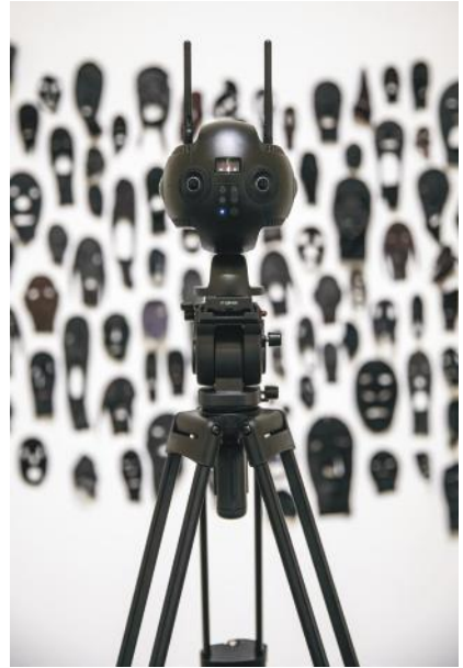
Image: A closer look at the Insta360 Pro 2, a 360 Virtual Reality (VR) camera used to create interactive virtual tours for CTSA.
