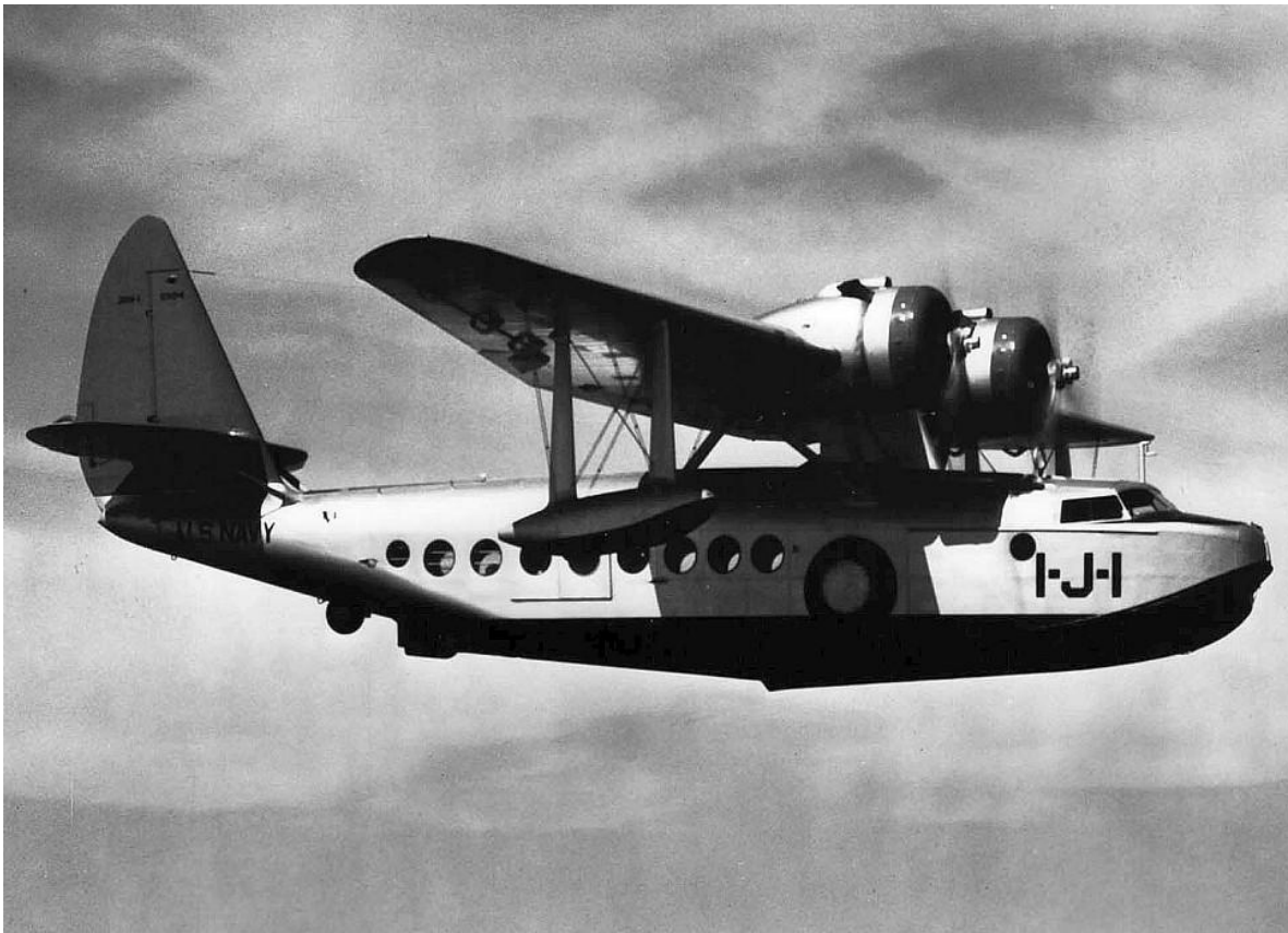
A photo of the National Air and Space Museum's Sikorsky JRS-1 in flight with Utility Squadron 1 (VJ-1) sometime between 1938 and 1941. VJ-1 used the Sikorsky JRS-1 for a variety of utility roles including transporting personnel and cargo, towing targets for anti-aircraft gunnery practice, and survey flights for aerial photography. (National Archives Photo)
