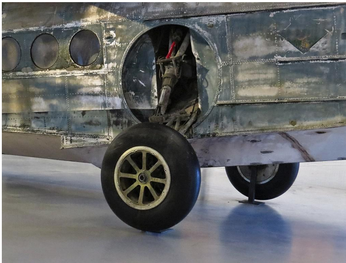
Close-up photo of the main landing gear of the Sikorsky JRS-1. In addition to being used to land and take off from conventional runways, the JRS-1 could, in theory, be taxied down a seaplane ramp into the water on its landing gear. Once in the water, the pilot would retract the landing gear before taking off.
