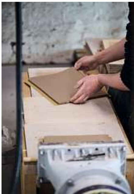
Below: The mixture is extruded, shaped and fired at 800 to 850°C in electric kilns, around 400°C lower than clay.
