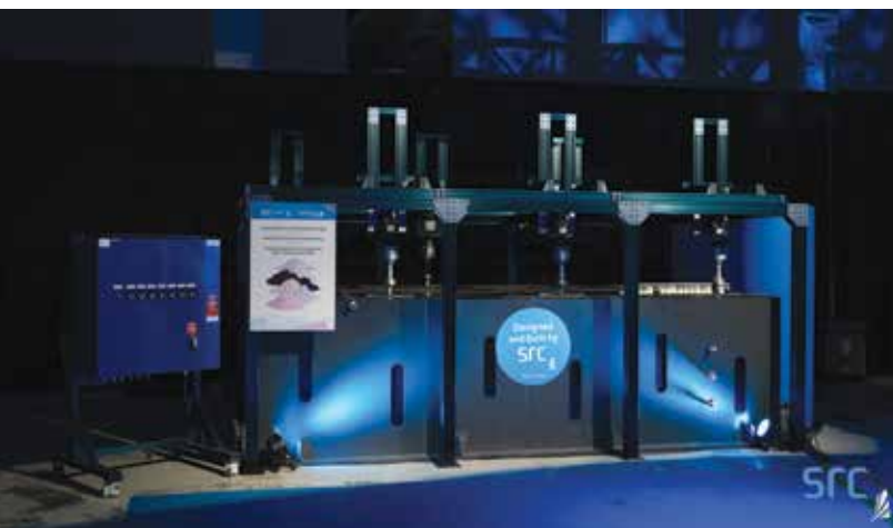
SRC designed and manufactured proprietary commercial-scale solvent extraction cells for its Rare Earth Processing Facility. All photos courtesy of SRC.
