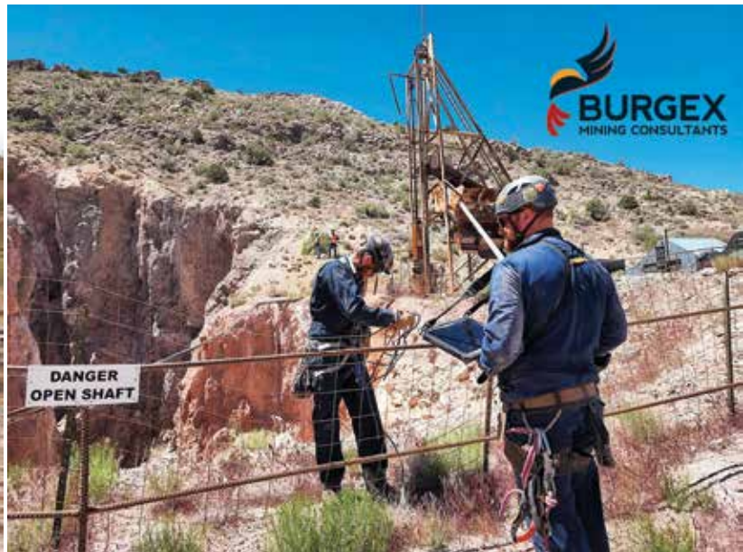
Burgex team members scanning Ares Lost Sheep Mine underground and open stope with a handheld LiDAR scanner.
