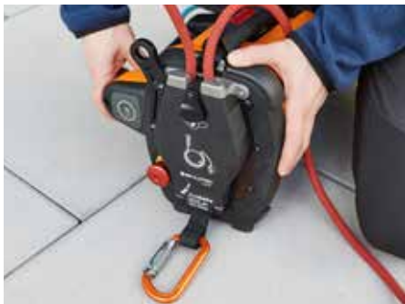
Semi-static working rope (SUPER STATIC 11.0) is placed in the ACX POWER ASCENDER
