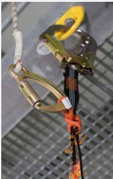
Rescue loop becomes visible when shock absorber is activated.
