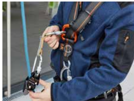
Backup rope is connected to the guided type fall arrester as per EN 353-2 and to the front attachment point of the harness
