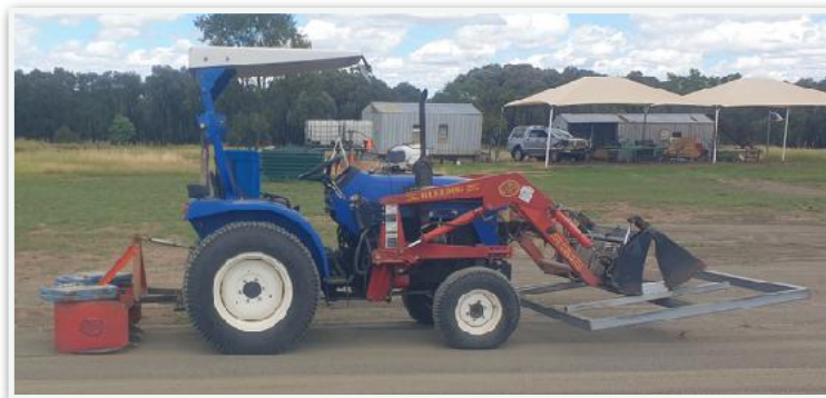
The Jinma Tractor with spreader and grader box
