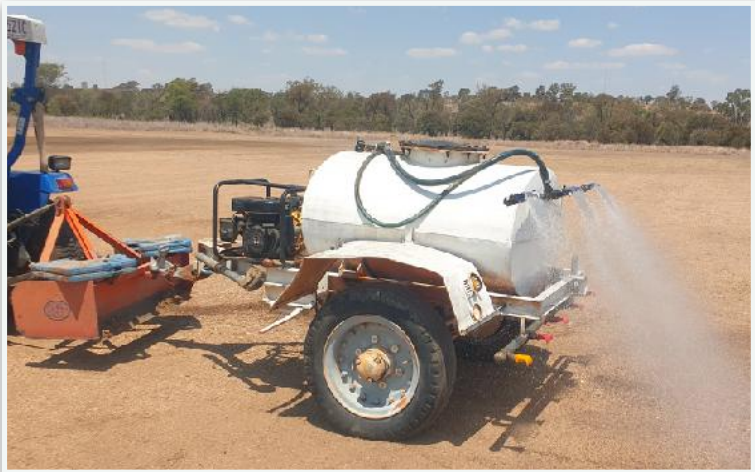
Our water/fire fighting trailer with pressurised spray
