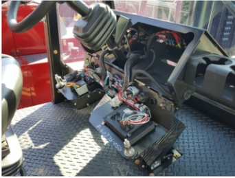
Flip-down Dash with Color/Number Coded Wiring (Standard)
