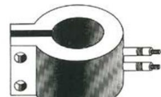
FULL BAND CONSTRUCTION WITH CLAMP LUGS
