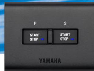
Twin Engine Start/Stop Switch
