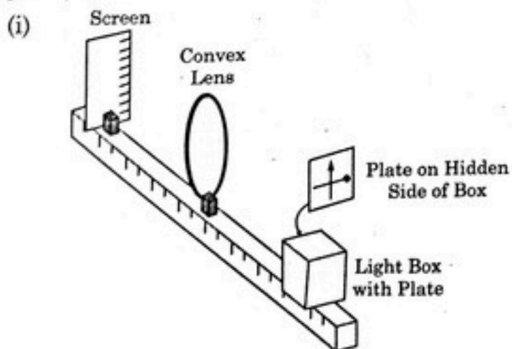
Consider the arrangement shown in figure. A black vertical arrow and a horizontal thick line with a ball are painted on a glass plate. It serves as the object. When the plate is illuminated, its real image is formed on the screen.
