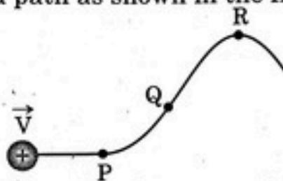
The path followed by the proton is always in the plane of the paper. What is the direction of the magnetic field in the region near points P, Q and R? What can you say about relative magnitude of magnetic fields at these points?
