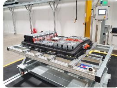
BMS & cover install
