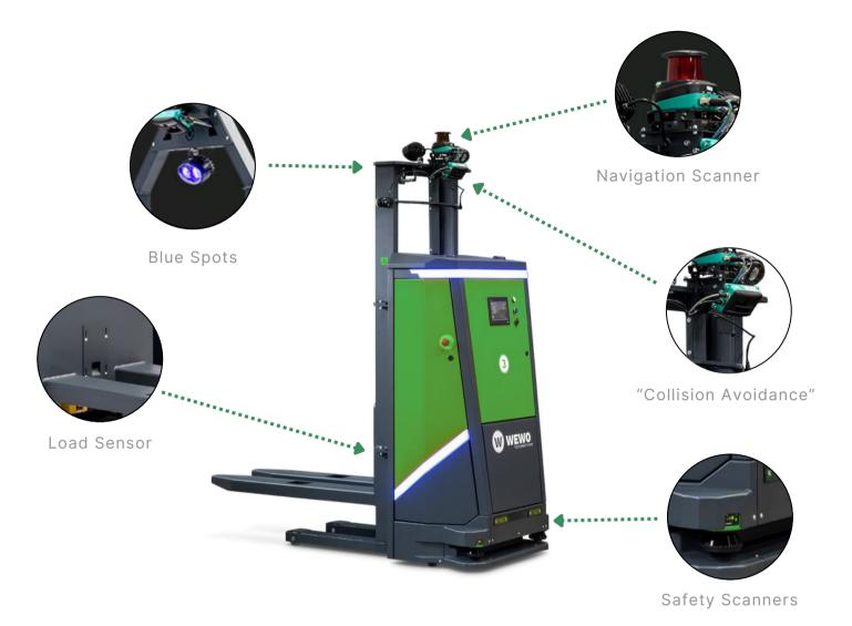
The AGVs are equipped with advanced safety systems designed to protect employees, infrastructure, and the robots themselves.
