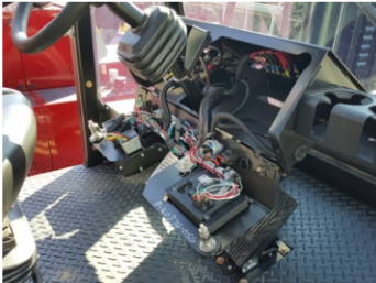
Flip-down Dash with Color/Number Coded Wiring (Standard)
