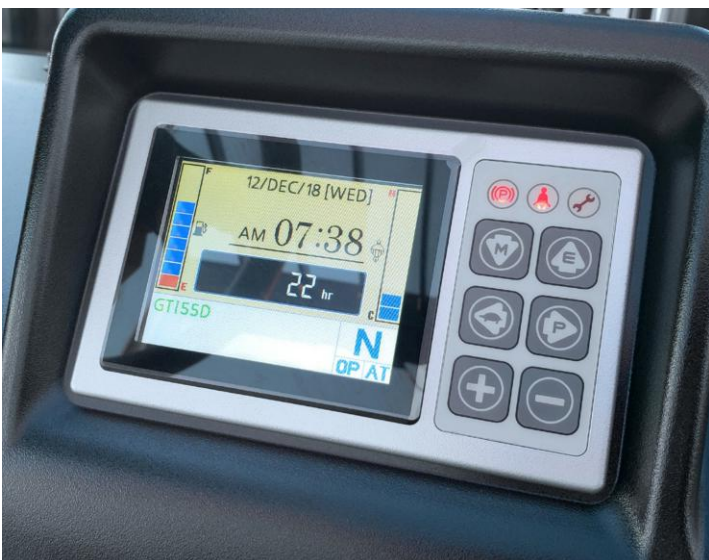
Weather Sealed High Visibility LCD Diagnostic Display Includes Fault Code Storage and is Password Protected
